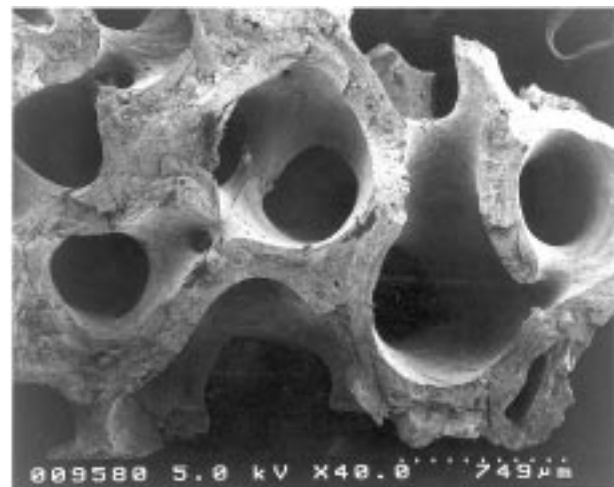
Figure 4 Scanning electron micrograph of a thin section of successfully defatted/hypochlorite-treated bovine bone matrix.
